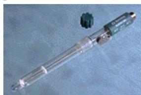
In the normal case the electrode should be filled with reference electrolyte  $c(\text{KCl})=3 \text{ mol/L}$ . The
