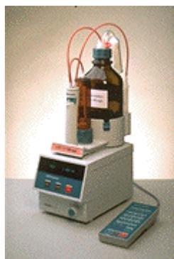
In the preparative laboratory, the DIS C mode is used for continuous dispensing. Two 665 Dosimats in tandem operation can be controlled via PC and thus allow uninterrupted dispensing. High accuracy of the dispensing and chemical resistance of the materials used allow universal deployment of the 665 Dosimat.
